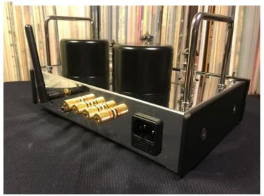
At the back of the device is the right side with an electrical input and a Bluetooth antenna in the front. Antenna included in the box content. Due to its circumferential extension, you experience problems such as breakage during connection. It supports the Bluetooth 4.0 standard and has aptX\_support. On the left side there is 1 RCA input, 1 3.5mm input, 1 USB input and subwoofer output.
